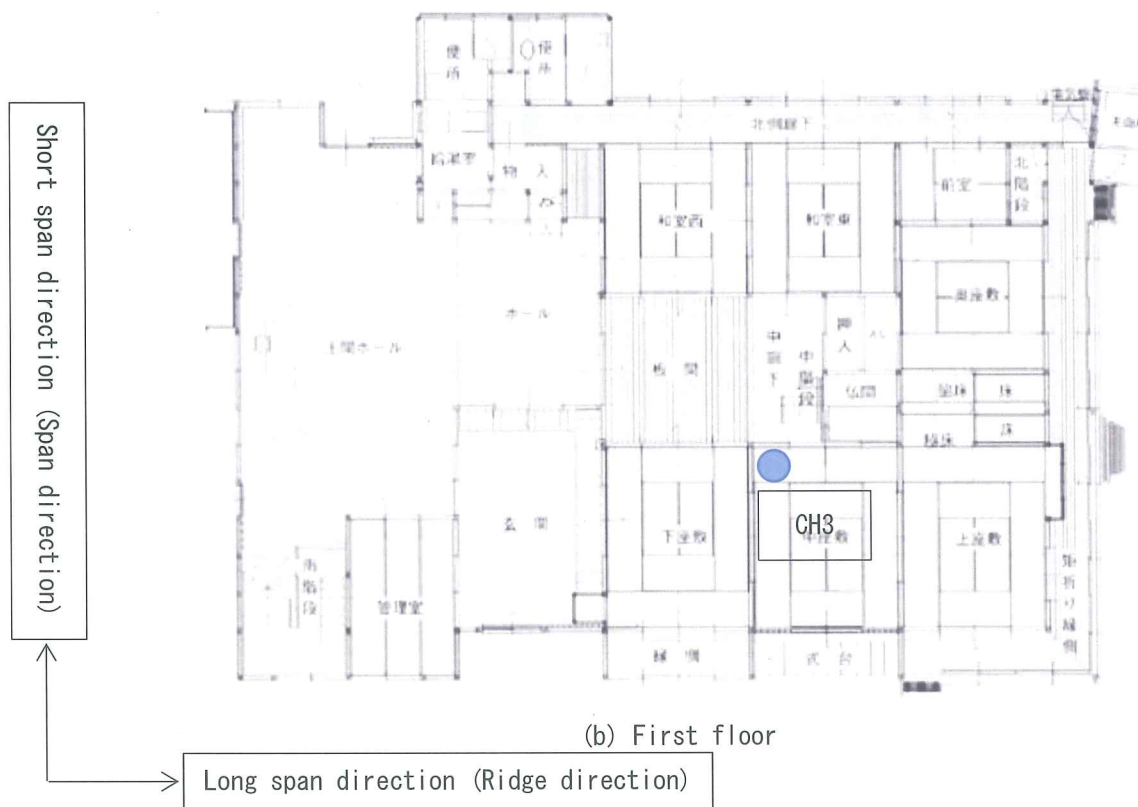
Fig.5 Oscillator and accelerometer installation in Ohkumo Memorial house
