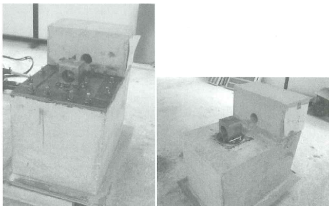
Photo 6 Pull-Out Test Models of Steel Anchor
