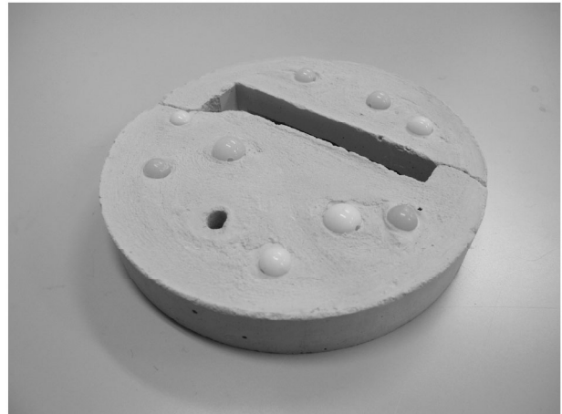
Fig.7 The cracked cement base
